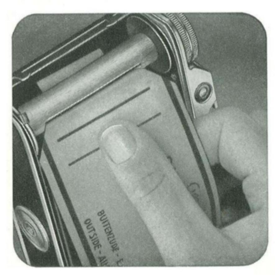
In this camera only filmspools can be used which have a thick core of metal or wood. These are marked on the packing of the spool with B II/8 or 120.
