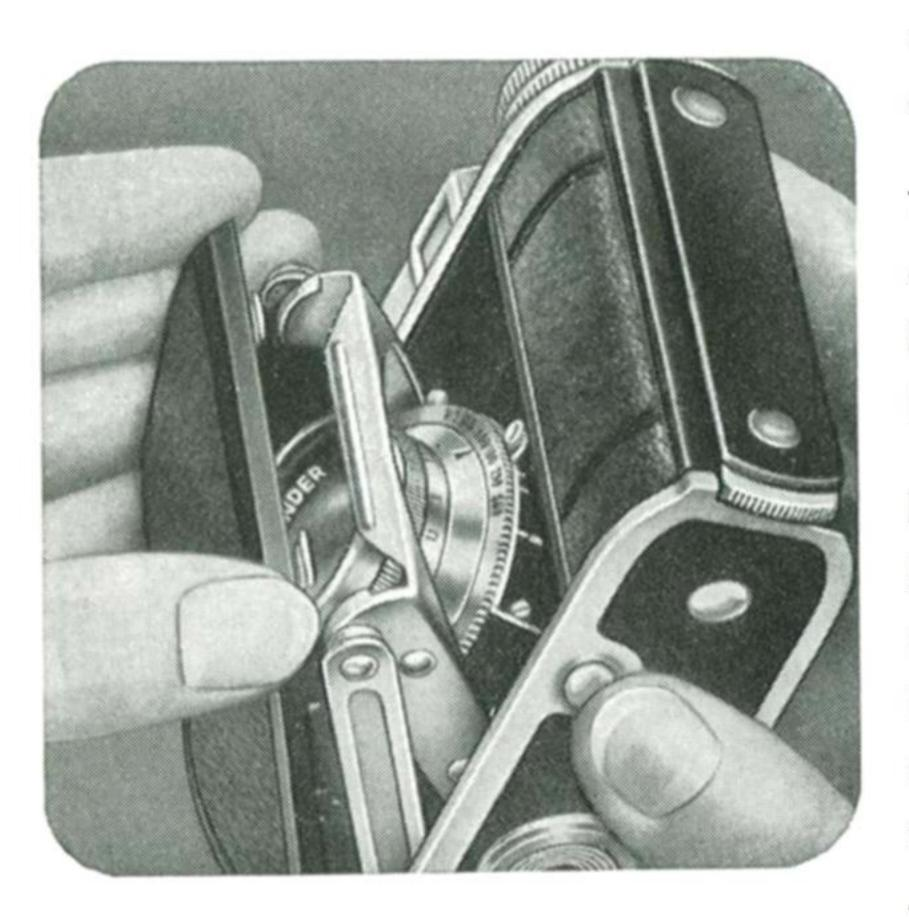
On depressing button 21 the camera front will open up. It is pulled down with thumb and index finger on both corners until the two struts 4 engage.
